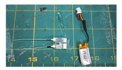
Dronetag offers a 50Mah LiPo and a charger all set to go to power the unit for an additional \$20 (or so, the price is in Euro's). I should have added that as my effort to wire a small LiPo failed and so I had to add a bigger battery.
